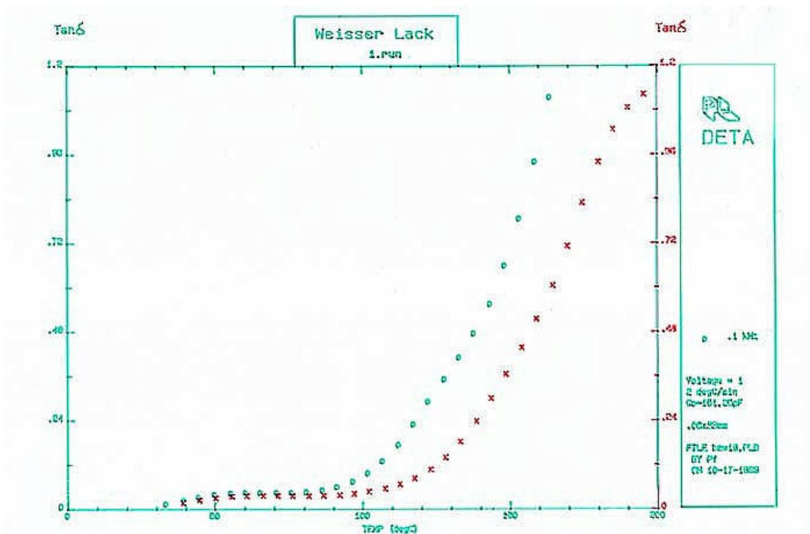
DETA is very sensitive for detecting moisture absorption at the interface and in the polymeric bulk material.
