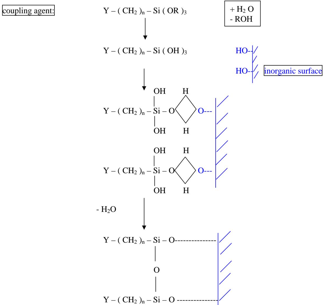
*Y can be an amino-, epoxy-, etc. group that is chemically incorporated into the adhesive.*
