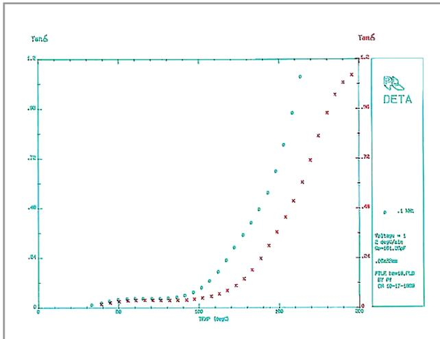
FIGURE 8 DETA of a composite cured at different temperatures
