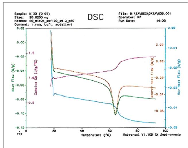
FIGURE 6 MDSC spectra of a typical epoxy matrix
