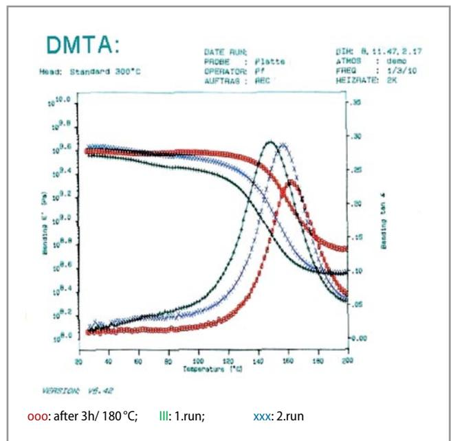
FIGURE 7 DMA curves at various crosslinking densities of an epoxy system
